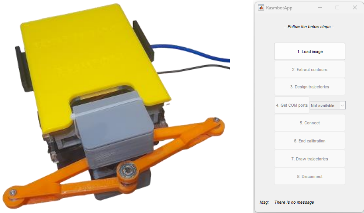
Fig. 5: The implemented robot: The left and right subfigures show the robot's device and its application UI.
